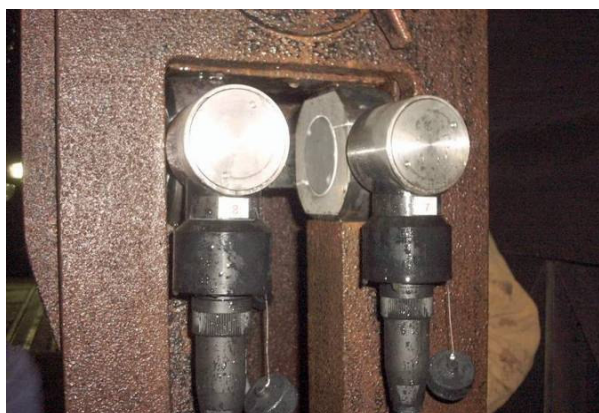
Photo 1. WPS-Ec inserts installed in connector for rope length change manufactured by RYFAMA
