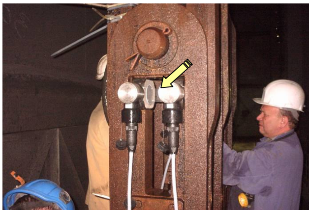
Photo 6. WPS-Ec inserts in the suspension of the vessel in 1.3 shaft
