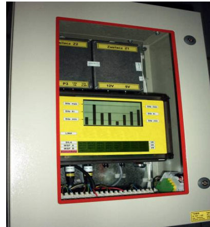
Photo 5. Visualization of the force level in the ropes on the stand for winches control ( F_{sr} + 5\% ; F_{sr} ; F_{sr} - 5\% )
